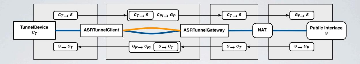
IP-layer packets get encapsulated as UDP payload for transmission over tunnel
